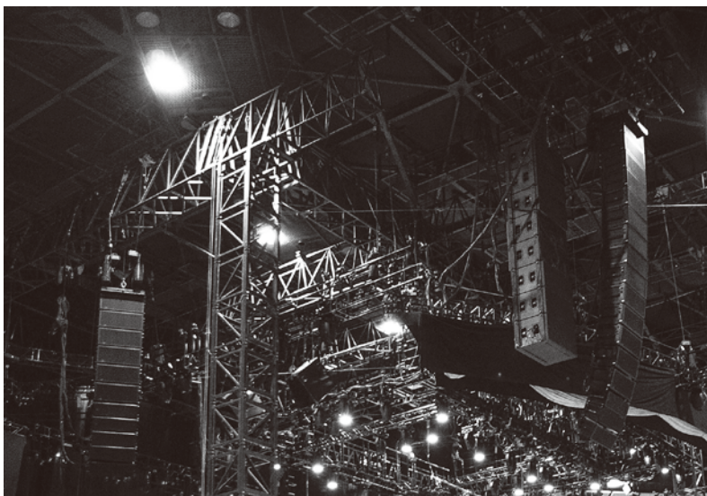
Flown speaker system consists of LEO-M, MICA, 700-HP
